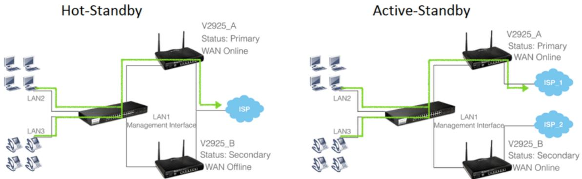
In Hot-Standby Mode, Primary and Secondary router share the same WAN source. Usually, only the Primary is online. When Primary goes down, Secondary comes up and use the same WAN line to dial up, and continue to provide Internet service to LAN clients.
