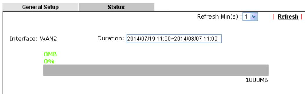
If the WAN budget is exhausted, a lock will be displayed on the page if Shutdown WAN interface is selected. Which means no data transmission will be carried out. Moreover, the system will send out a warning message to the administrator if Mail Alert is selected. Or, the system will send out SMS message to the administrator if SMS message is selected.
