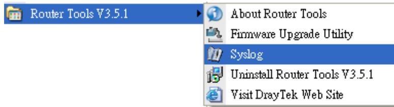
3. In the Syslog application, select the router you wish to monitor. Remember to select the network adapter to be used to connect to the router under Network Information, or else Syslog traffic cannot be received from the router.
