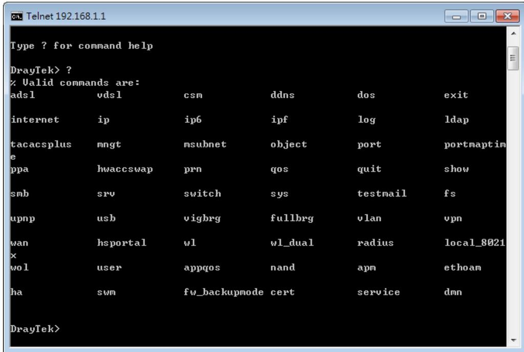
For users using previous Windows system (e.g., 2000/XP), simply click Start >> Run and type Telnet 192.168.1.1 in the Open box as below. Next, type admin/admin for Account/Password. And, type ? to get a list of valid/common commands.
