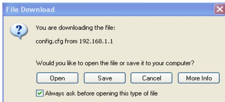
The configuration will download automatically to your computer as a file named config.cfg. The above example is using Windows platform for demonstrating examples. The Mac or Linux platform will appear different windows, but the backup function is still available.
