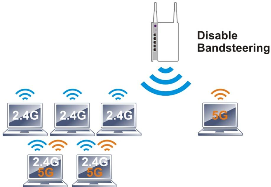
If a dual-band client is detected, the AP will let the wireless client connect to the less congested wireless band, such as the 5GHz band, to reduce network congestion.
