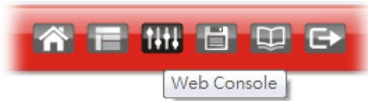
It is not necessary to use the telnet command via DOS prompt. The changes made by using web console have the same effects as modified through web user interface. The functions/settings modified under Web Console also can be reviewed on the web user interface.
