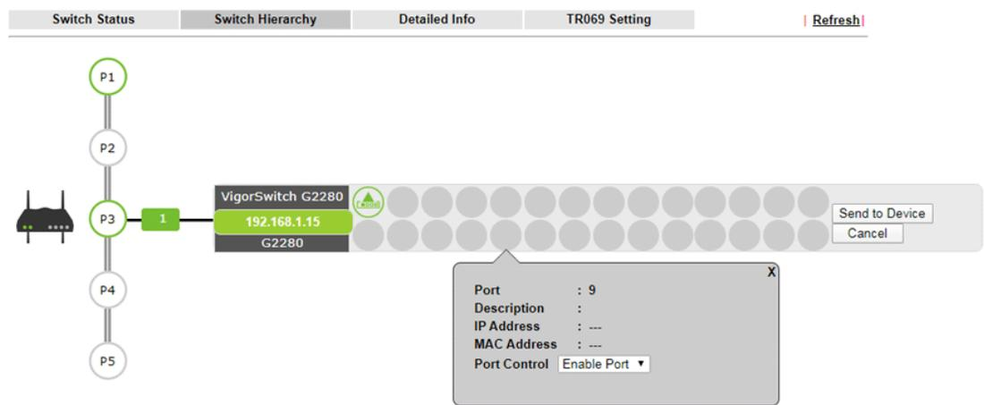
Please note that, Shutdown Port is available for LAN port of VigorSwitch connects to a LAN device. When it is checked, after clicking OK, the network connection between that device and VigorSwitch will be terminated.
