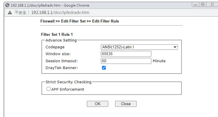
Codepage - Sets the codepage used by the URL content filter to match URLs against keywords in profiles. Choosing the appropriate codepage can increase the accuracy of the URL Content Filter. The default value is ANSI 1252 Latin I. If the setting is None, no decoding of URL will be performed. If you are unsure of which codepage to use, please start the Syslog application, and the recommended codepage will be shown in the Codepage Information tab in the Setup dialog box.
