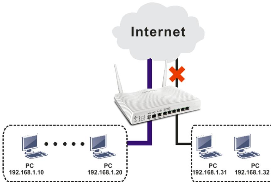
The way we can use is to set two rules under Firewall. For Rule 1 of Set 2 under Firewall>>Filter Setup is used as the default setting, we have to create a new rule starting from Filter Rule 2 of Set 2.
