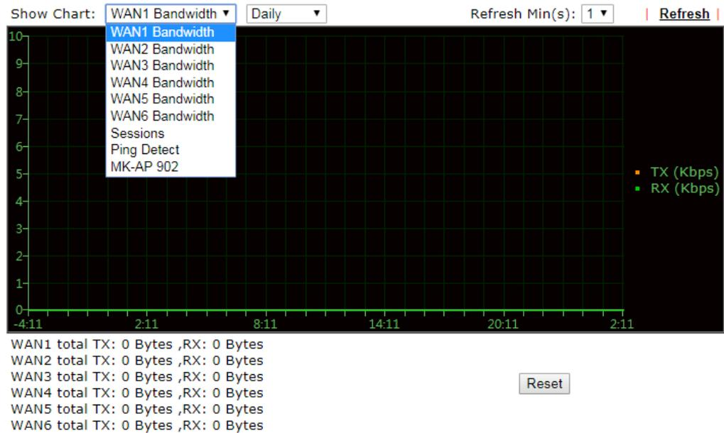
The horizontal axis represents time. Yet the vertical axis has different meanings. For WAN1/WAN2/WAN3/LTE/WAN4/WAN5/WAN6 Bandwidth chart, the numbers displayed on vertical axis represent the numbers of the transmitted and received packets in the past.
