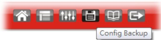
There is one way to store current used settings quickly by clicking the Config Backup icon. It allows you to backup current settings as a file. Such configuration file can be restored by using System Maintenance>>Configuration Backup.
